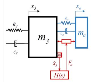
Scheme of a hybrid tuned mass damper from "Robust hybrid mass damper". Collette, Chesné, JSV (2016)
